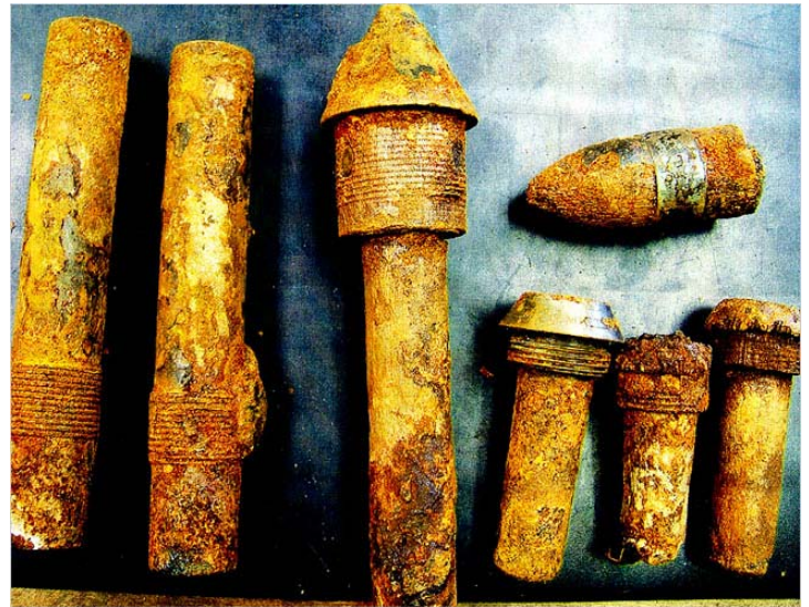
U.S. MILITARY FUSES AND ADAPTORS FOUND ON LONG BEACH ISLAND, NEW JERSEY – SOME CONTAINING UNEXPLODED GUN POWDER (PHOTOGRAPHY BY U.S. ARMY CORPS OF ENGINEERS)
